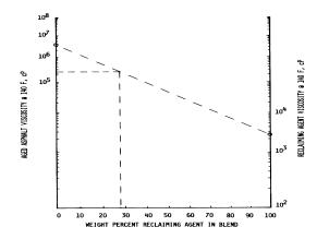
Figure 1, Nomograph for Viscosity.
